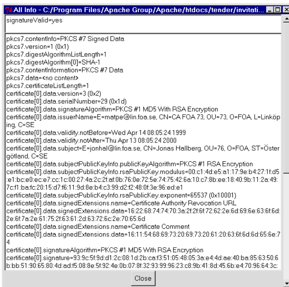
Figure 4: Pretty print of the PKCS #7 object displayed by the designed user interface.
